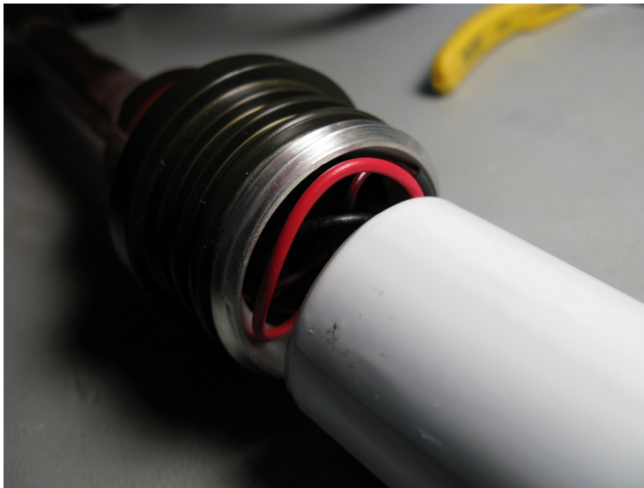
Figure 5. Wiring in danger of pinching. Take great care not to allow wires to be pinched during assembly! If this red (power) wire is pinched when the battery housing is secured, it could short out the battery pack, leading to instrument failure, battery leakage, and permanent damage to the housing.
