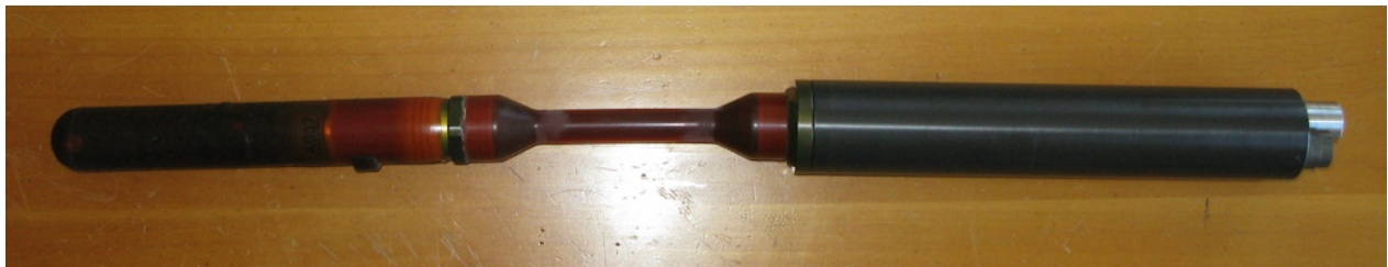
Figure 1. Model B003A Acousonde assembled with B003-XHD external battery housing.
