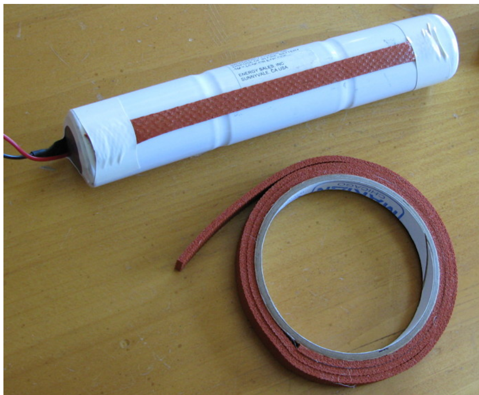
Figure 3. Example of mechanically securing battery pack using a silicone foam strip. If it appears the battery pack may move excessively within the housing, tape foam to the side of the pack before inserting into the housing. In this example, a length of silicone foam about half the length of the pack was stretched out to the pack’s full length and affixed to the pack using electrical tape.
