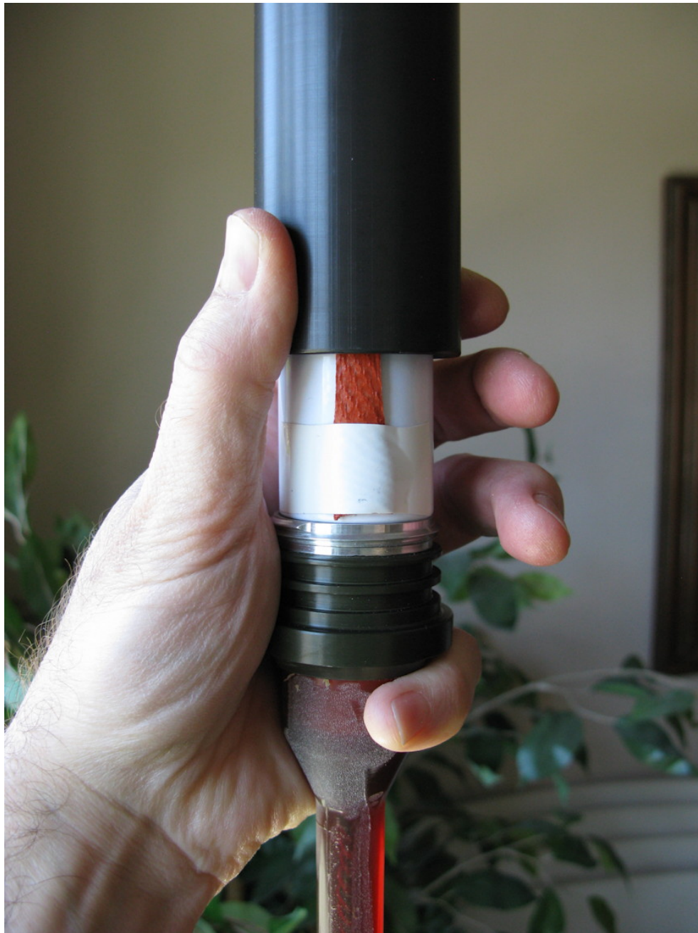
Figure 6. Avoiding wire pinch during assembly. To avoid wire pinch, balance the battery pack vertically on top of the bulkhead during assembly while lowering the housing onto the pack. This way no wiring will become exposed to pinching as the housing is assembled. Take care to keep the o-rings clean during this process (the o-rings are not shown in this photograph).
